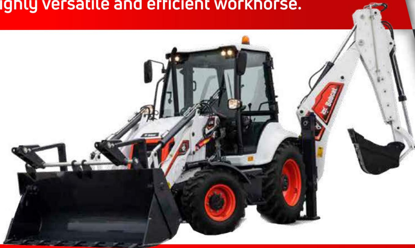
Bobcat Rental's TLB is also another popular and adaptable machine. It is being used for digging, trenching, breaking, or general materials-handling.
